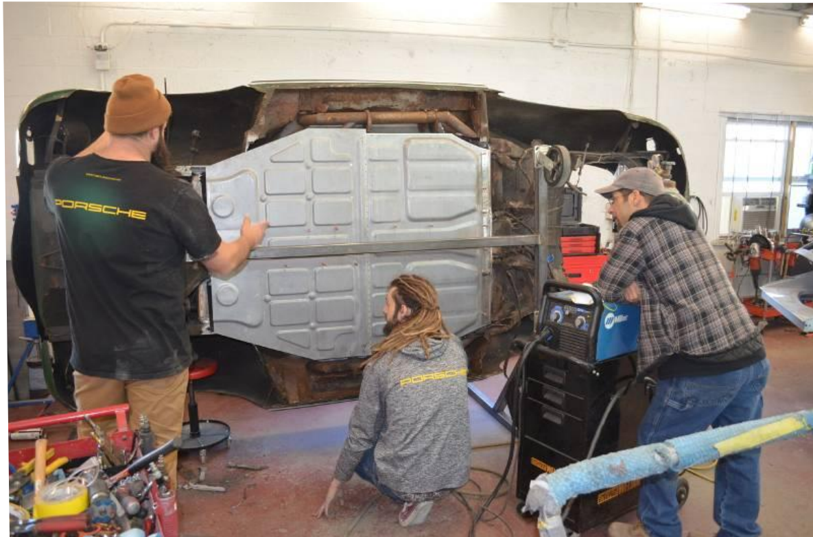
Ryan Kenton, Ryan Gill, and Troy Smith discuss the new floor pan installation on the Simone 356 Cab
